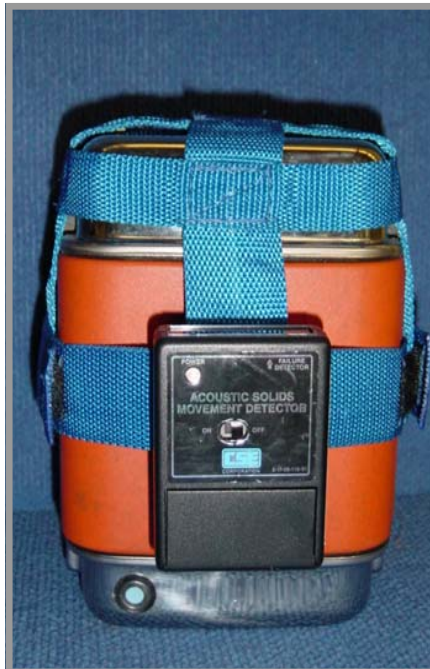
Acoustic Solids Movement Detector Mounted on a SR-100
